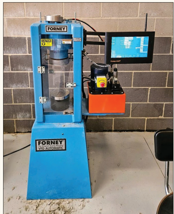
Figure 1: Cylinder Compression Testing Machine at the Triangle Ready Mix Testing Lab
